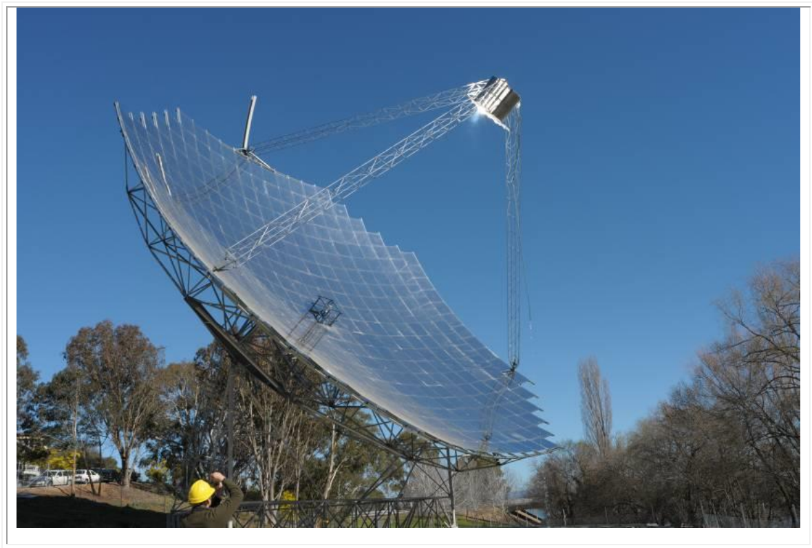
Fig. 11. First on sun tests with all mirrors uncovered
