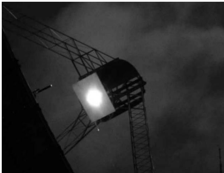
Fig. 10. Zoomed in view of the flux mapping target through neutral density filters.
