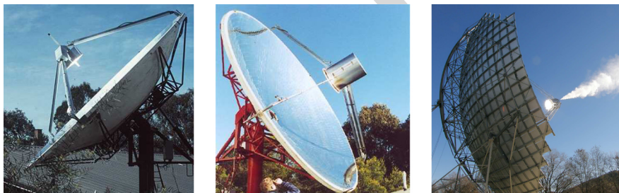
Fig. 3. Left: 20-m 2 dish concentrator with the Mark II prototype receiver—here the receiver is external to the casing. Center: 20-m 2 dish concentrator with 15-kW chem ammonia receiver—here the receiver is within the casing. Right: 489-m 2 dish on sun (test run with steam vented to atmosphere). (Photos: ANU.)
